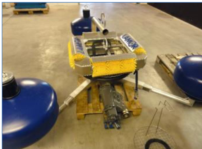
Figure 47 Typical Offshore Recovery Device with Brush Attachment.
