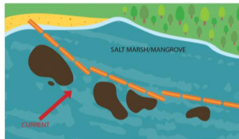
CASCADE BOOMING Deflects oil away from sensitive resources to a point of enhanced natural collection for recovery.
