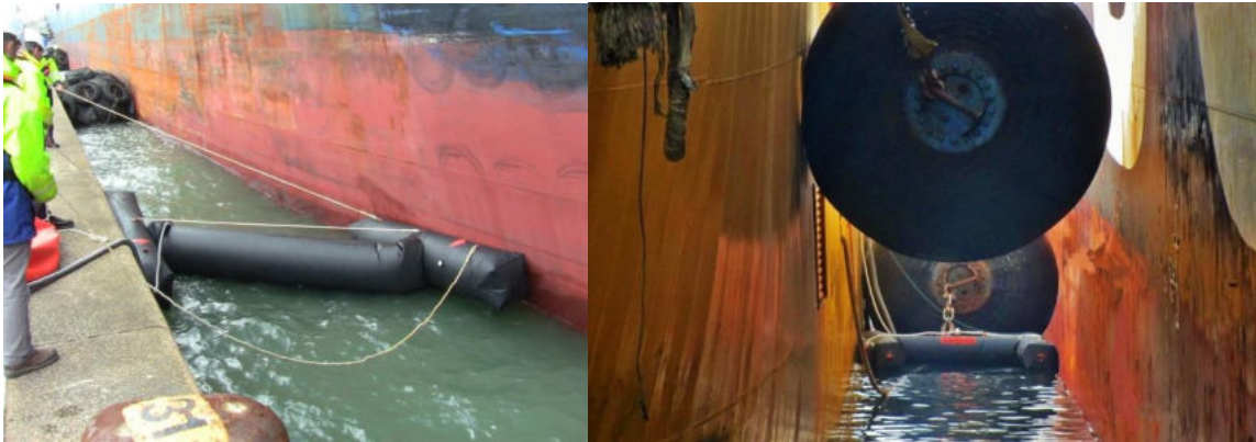
Figure 43 Inflatable H booms deployed between vessel and dockside and between two vessels.
