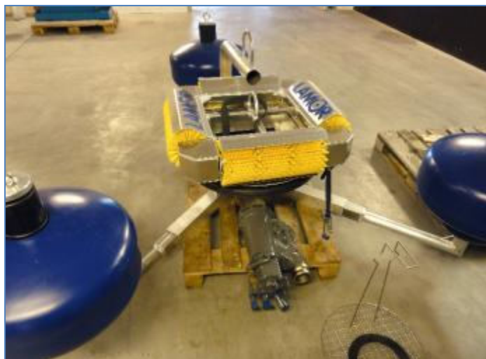
Figure 47 Typical Offshore Recovery Device with Brush Attachment.
