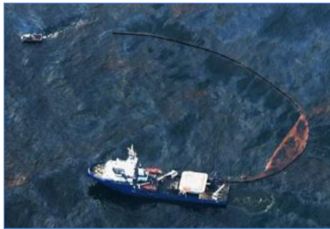
Figure 46 Offshore Containment and Recovery J Formation.
