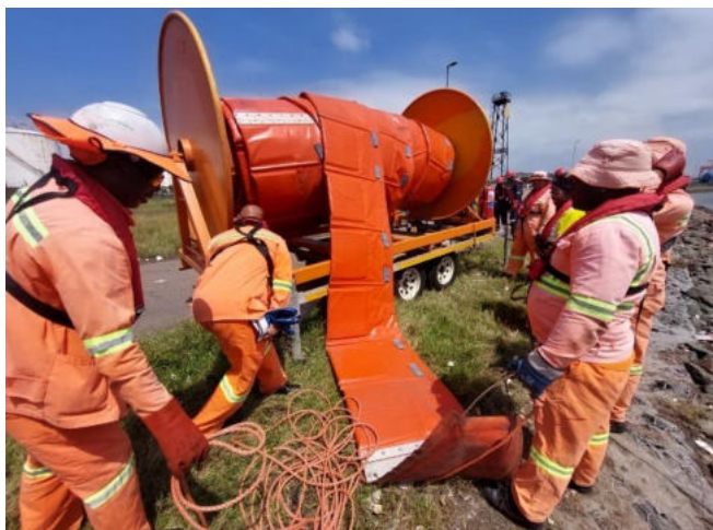
Setting Up Fence Boom
