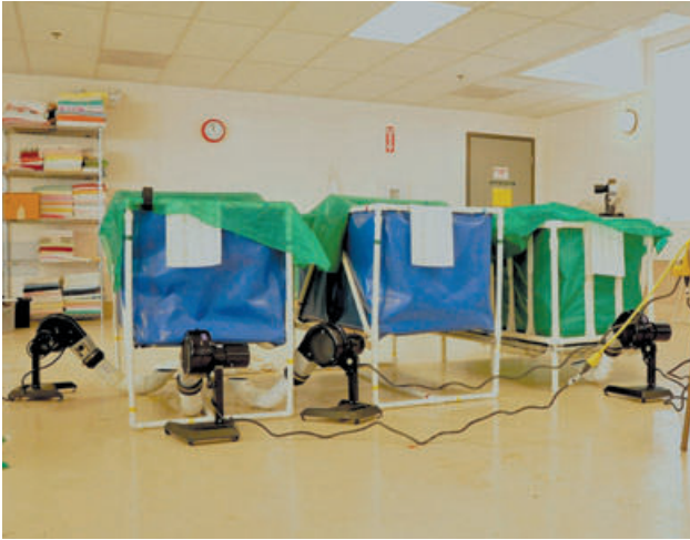
Animals that need to be dried after cleaning are placed into net-bottomed pens and warmed with air from external fans.
