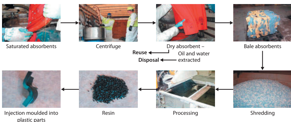
Figure 7 Illustration of a recycling process from boom material to plastic products
