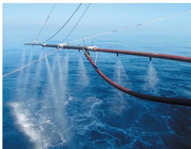
Dispersant spraying from a vessel-mounted spraying arm.
