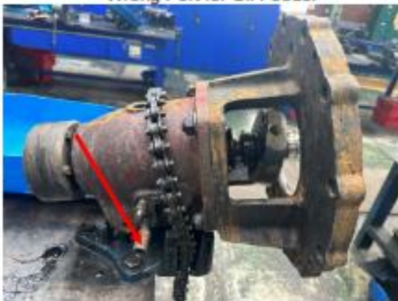
Wrong Port for Oil Feeder
