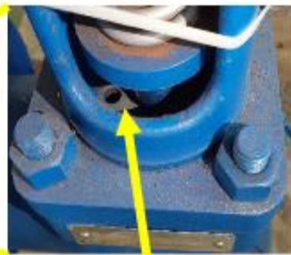
Drain/vent hole: d=10.3mm
