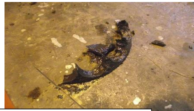
Failed ball bearing cage
