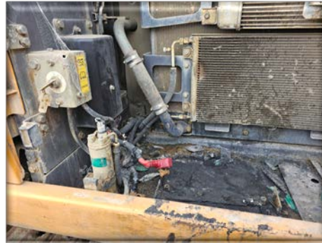
Battery Compartment of Excavator (battery acid splash mark on aircon radiator)
