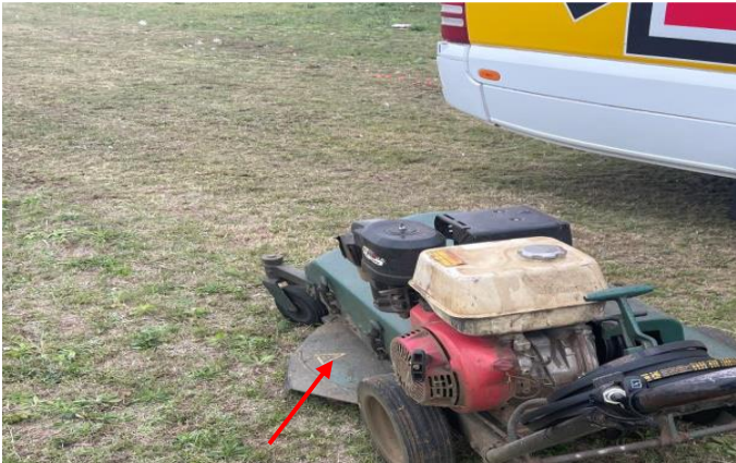
Outlet/chutes face at an angle towards the back of the machine and not directly away from the operator
