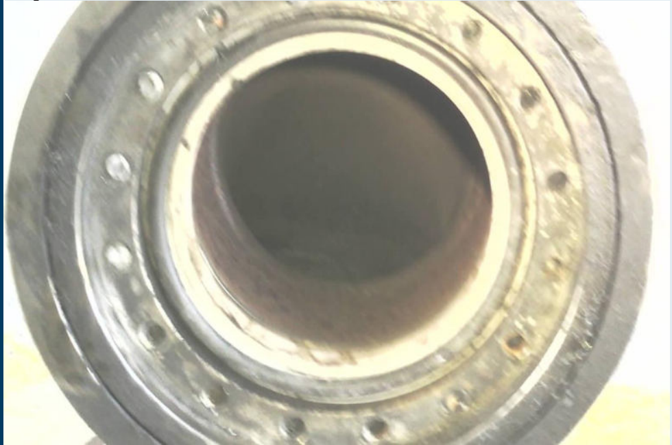
Flange from swivel where bolts shreaded off
