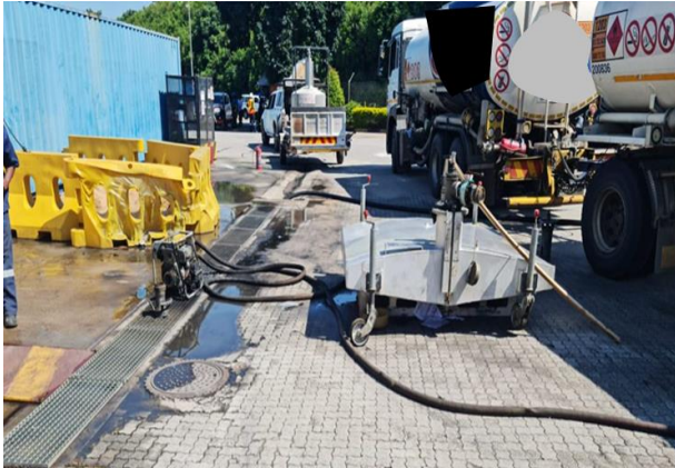
Picture 1: Meter Calibration rig after the fire still connected to the truck
