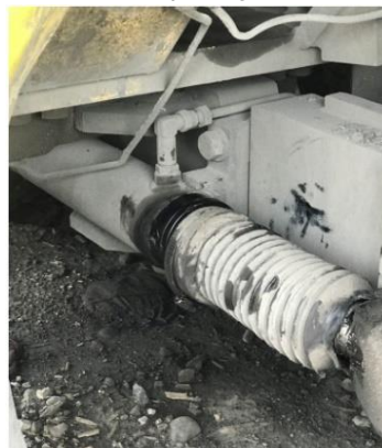
Oil Leak in Steering Cylinder
