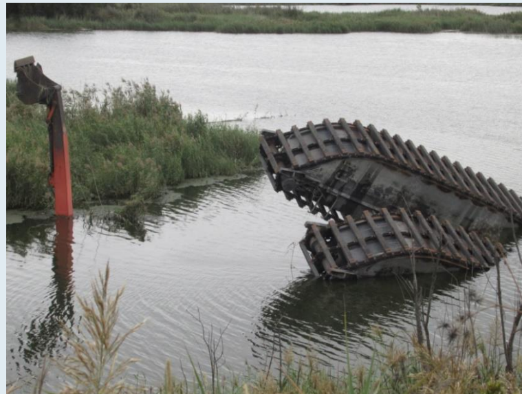
The amphibious excavator after it capsized at outside ash fine coal dam
