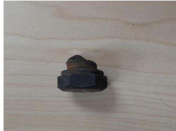
Top view of dislodged plug
