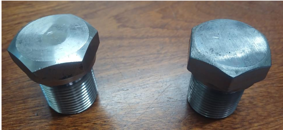
Stainless steel left and carbon steel on right
