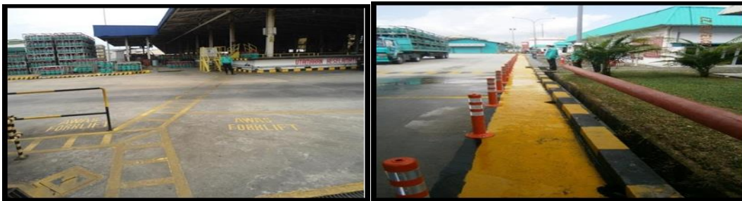
Figure 2: Example of pedestrian walkway with clear marking
